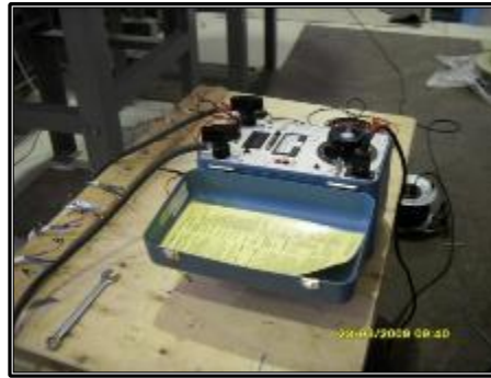
Testing of contact resistance
